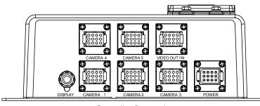
Controller Connections Refer to the CV5500M Quick Installation Guide for Detailed Wiring Information and Connector Arrangement
